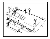
Replace the Fuse of PU1.
